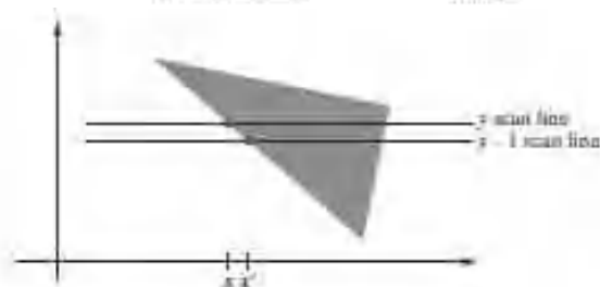
FIGURE 6 Scan lines intersecting a polygon surface.
