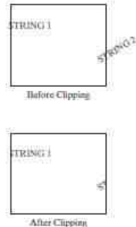
FIGURE 33 Text clipping performed on the components of individual characters.
