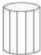
FIGURE 7 Wire-frame representation for a cylinder, showing only the front (visible) faces of the polygon mesh used to approximate the surface.
