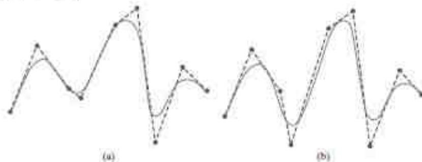
FIGURE 28 Local modification of a B-spline curve. Changing one of the control points in (a) produces curve (b), which is modified only in the neighborhood of the altered control point.
