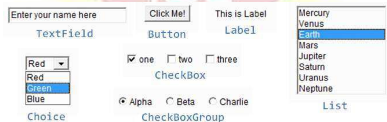
Figure: AWT Controls
