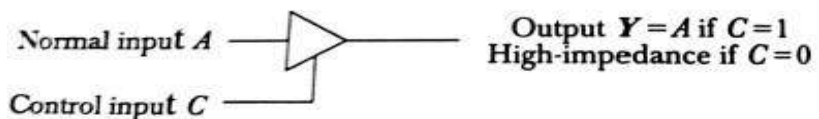
Figure 4-4 Graphic symbols for three-state buffer.
