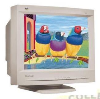
CRT monitors are based on the cathode ray tubes. They are like vacuum tubes which produce images in the form of video signals. Cathode rays tube produces a beam of electrons through electron guns that strike on the inner phosphorescent surface of the screen to produce images on the screen. The monitor contains millions of phosphorus dots of red, green and blue color. These dots start to glow when struck by electron beams and this phenomenon is called cathodoluminescence.
