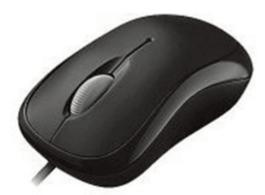
An optical mouse uses optical electronics to track its movement. It is more reliable than a mechanical mouse and also requires less maintenance. However, its performance is affected by the surface on which it is operated. Plain non-glossy mouse mat should be used for best results. The rough surface may cause problems for the optical recognition system, and the glossy surface may reflect the light wrongly and thus may cause tracking issues.
