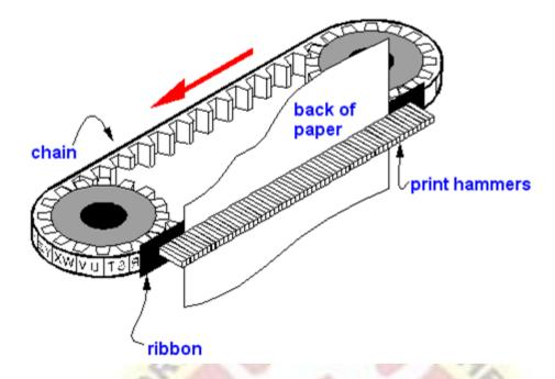
Chain printer is a line printer that uses a rotating chain to print characters. The characters are embossed on the surface of the chain. The chain rotates horizontally around a set of hammers, for each print location one hammer is provided, i.e., the total number of hammers is equal to the total number of print positions.
