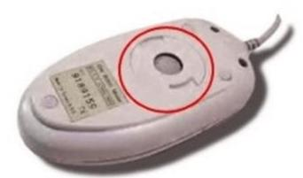
It has a system of a ball and several rollers to track its movement. It is a corded type of mouse. A mechanical mouse can be used for high performance. The drawback is that they tend to get dust into the mechanics and thus require regular cleaning.
