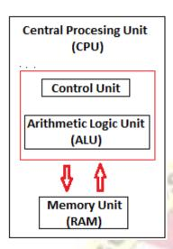
Control Unit: It is the circuitry in the control unit, which makes use of electrical signals to instruct the computer system for executing already stored instructions. It takes instructions from memory and then decodes and executes these instructions. So, it controls and coordinates the functioning of all parts of the computer. The Control Unit's main task is to maintain and regulate the flow of information across the processor. It does not take part in processing and storing data.
