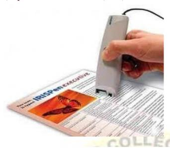
OCR computer input device is designed to convert the scanned images of handwritten, typed or printed text into digital text. It is widely used in offices and libraries to convert documents and books into electronic files.
