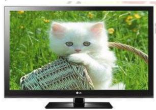
The LCD monitor is a flat panel screen that is compact and light-weight as compared to CRT monitors. It is based on liquid crystal display technology which is used in the screens of laptops, tablets, smart phones, etc. An LCD screen comprises two layers of polarized glass with a liquid crystal solution between them. When the light passes through the first layer, an electric current aligns the liquids crystals. The aligned liquid
