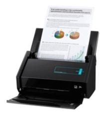
In this scanner, the document is inserted into the slot provided in the scanner. The main components of this scanner include the sheet-feeder, scanning module, and calibration sheet. The light does not move in this scanner. Instead, the document moves through the scanner. It is suitable for scanning single page documents, not for thick objects like books, magazines, etc.
