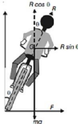
Fig Bending of a cyclist in a curved road
