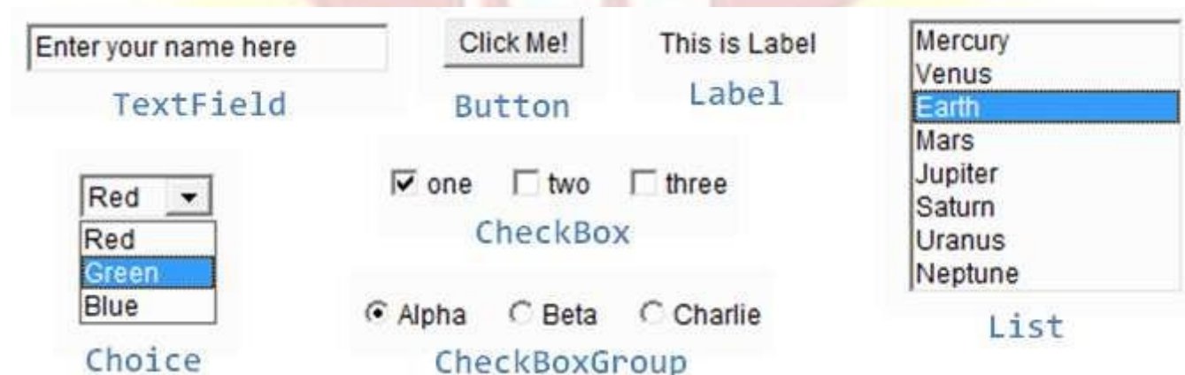
Figure: AWT Controls
