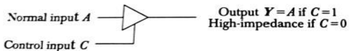
Figure 4-4 Graphic symbols for three-state buffer.
